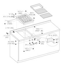
A: When installing with appliance cover, take the deeper cut-out into consideration (observe separate planning notes)
