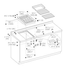
A: When installing with appliance cover, take the deeper cut-out into consideration (observe separate planning notes) B: 5¼° (133 mm) in the area of the cable clamp (left, on the rear side) C: ½° (3.5°)
