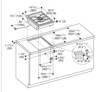
Minimum countertop thickness 1 3/16" (30 mm) for flush installation.
