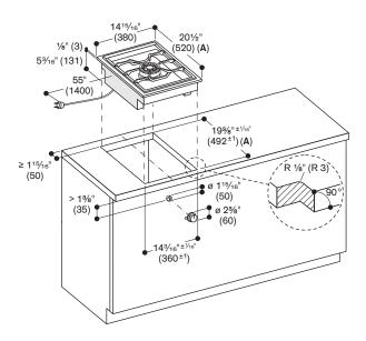
Minimum countertop thickness 3/4" (20 mm) for surface mounted installation.
