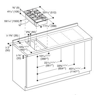
Minimum distance from the appliance cut-out to the side wall  $11^{13}/_{18}$ " (300 mm).
