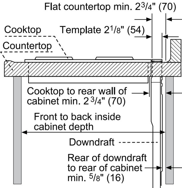
measurements in inches and (mm)
