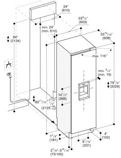
The maximum door front dimensions are based on a clearance of (3mm).
