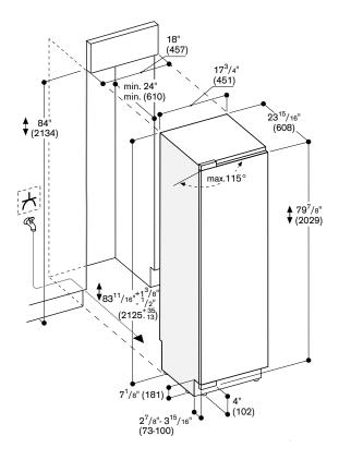
The door face dimensions are designed for a maximum gap of 1/8" (3 mm).
