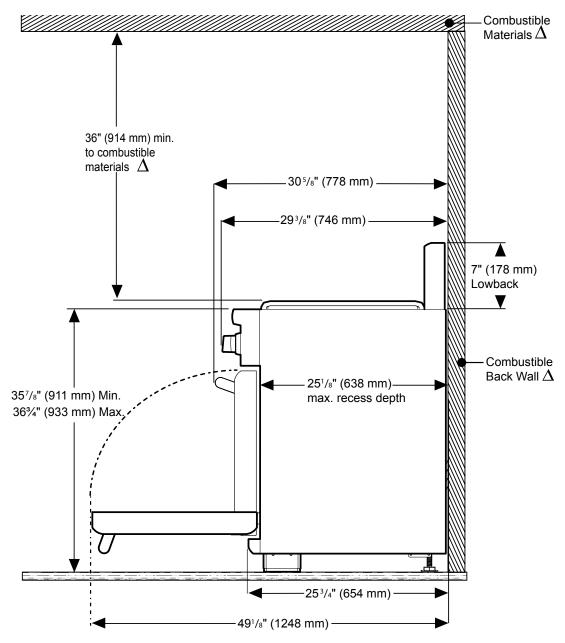
$\Lambda$  As defined in the "National Fuel Gas Code" (ANSI Z223.1, Current Edition). Clearances from non-combustible materials are not part of the ANSI Z21.1 scope and are not certified by CSA. Clearances of less than 6" (152 mm) must be approved by the local codes and/or by the local authority having jurisdiction.
