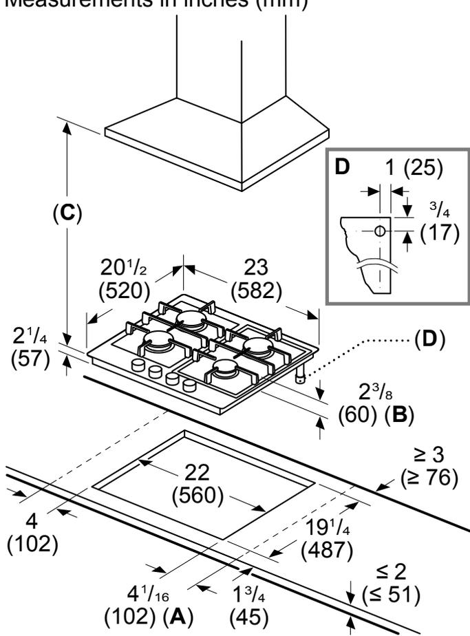
**A:**  $5\frac{1}{16}$ " (129 mm) required when installed with a built-in oven
