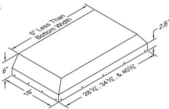
The VP521 transition is available for top vent applications at an additional charge.
