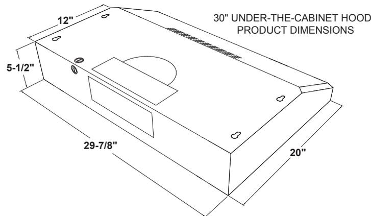
Exhaust outlet connects to 3-1/4" x 10" rectangular duct. Vent top or rear. Includes rectangular damper.
