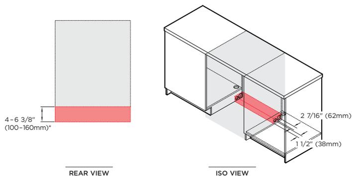
Service outlet at rear extends both sides, hoses and cords can be routed to either or both sides.
