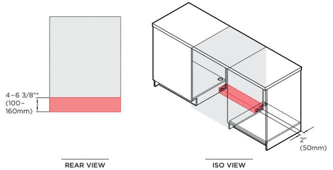
Service outlet at rear extends both sides, hoses and cords can be routed to either or both sides.
