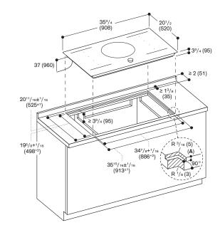
Minimum countertop thickness 1  $3/16\ensuremath{^{"}}$  (30 mm) for flush installation
