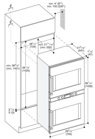
\* 8" (200 mm) clearance needed when using the pull-out system accessory BA 018 165
