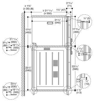
A: Only required if the water hoses for the BS steam oven cannot be accommodated in the corner recesses of the appliances.
