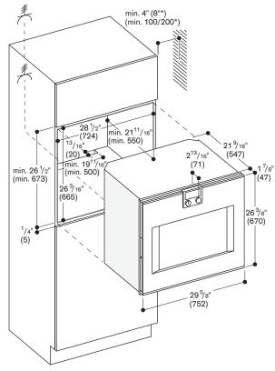
\* 8" (200) is minimum distance requirement in order to use pull-out system BA 018 105 and when installed wth handle.
