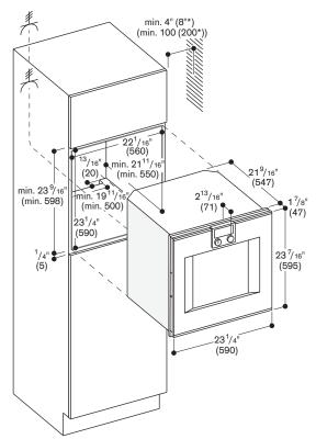
\* 8" (200) is minimum distance requirement in order to use pull-out system BA 016 105 and when installed with handle.
